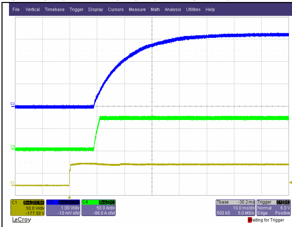
Start-up from Input Voltage Application at Full Load. Ch. 1: Vin Ch. 3: Vo Ch. 4: Io Load
